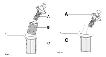
3. Turn the handle about 1/4 a turn anticlockwise and remove.
